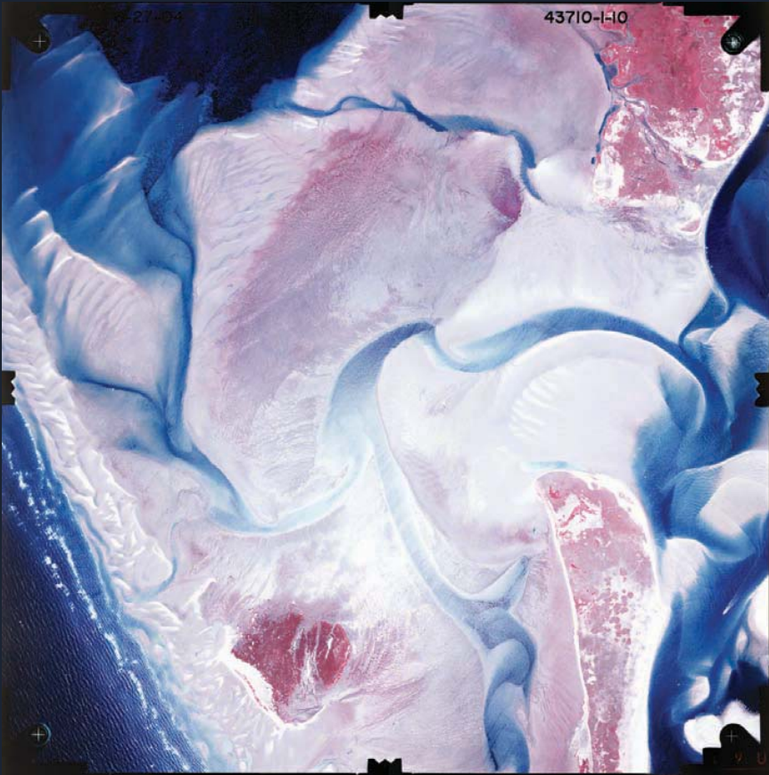
Color infrared aerial photograph (1:12,000) of a Cape Cod estuary for the U.S. Fish & Wildlife for use in aquatic vegetation studies
