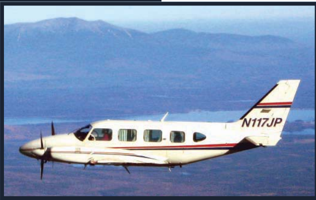
Piper Navajo twin-engine aircraft on an aerial mapping flight mission for Sewall near Mount Katahdin, Maine
