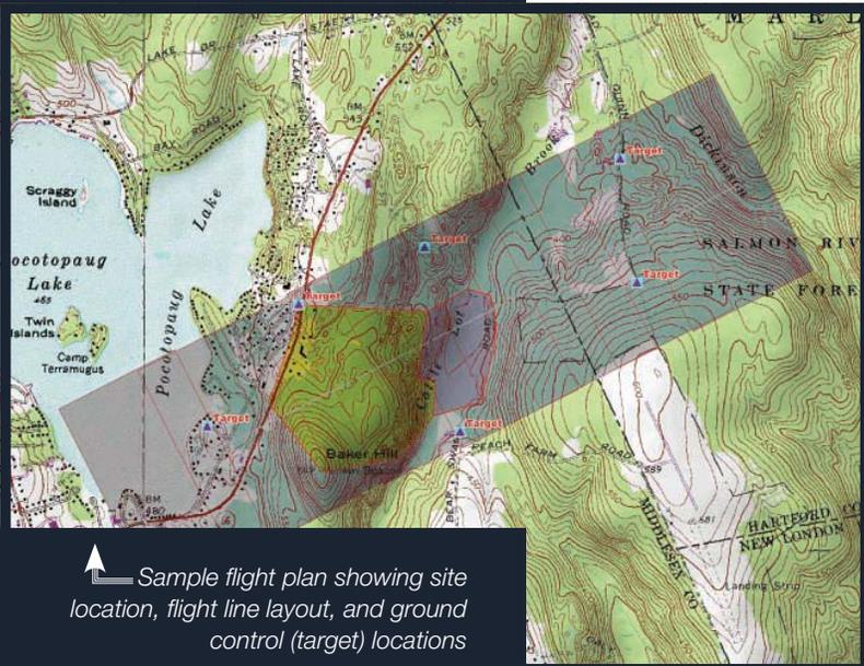
Sample flight plan showing site location, flight line layout, and ground control (target) locations
