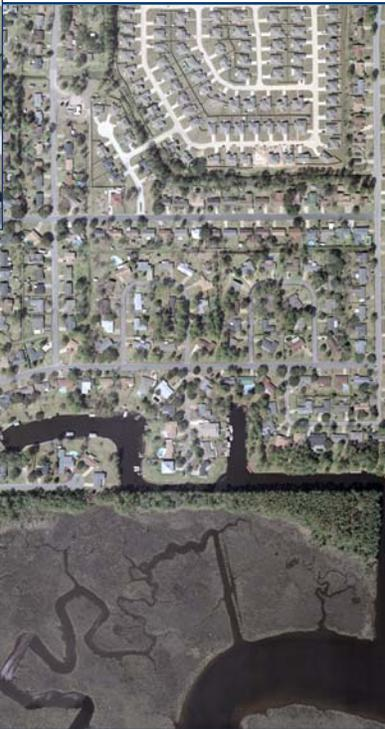
To ensure the orthophotography was suitable for the variable land use density in the County, Sewall flew the project area at three different photography scales (1"=3200', 1"=1200', and 1"=600') and applied a combination of IMU, airborne GPS, and softcopy aerial triangulation at the appropriate scales to update the existing DTM. This innovative approach enabled the County to balance high-accuracy requirements with significantly lowered costs.
