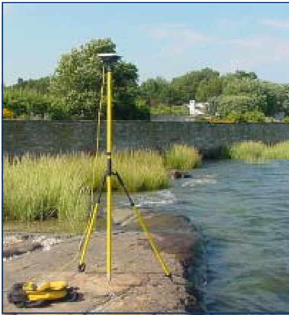
Rapid static GPS for controlling coastal topographic mapping.
